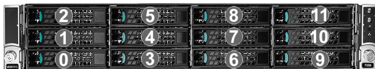
Figure 1-1 Velocity 7330 Appliance compute node front panel disk slot assignments
