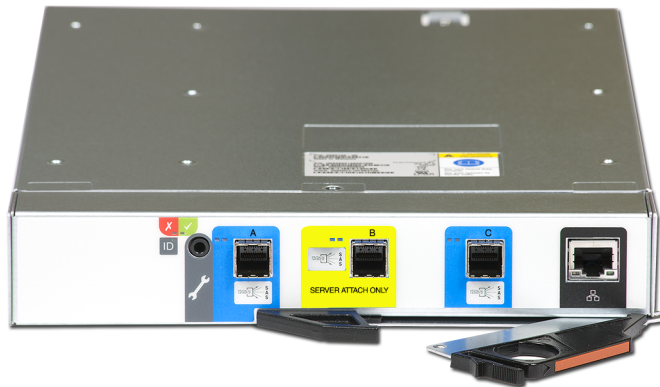
Figure 2-19 Veritas 5U84 Expansion Storage Shelf Expansion I/O module
