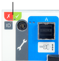
Figure 2-21 Expansion I/O module Status indicator LED location
