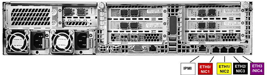
Figure 1-8 NetBackup 5340 Appliance rear port color codes
